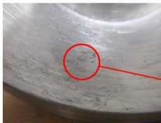
Small dents on the surface caused by cavitation
