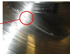
Rotor cracked by cavitation
