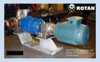
Molten Sulfur is burned to produce S02 in a process that conditions flue gas in coal burning power plants. A ROTAN® model MD101EFDK-1U33 was used as a transfer pump and another order followed in the same service. Specialized diaphragm metering style pumps deliver sulfur to the process at very low flow rates. (.19 to .42 gpm).
