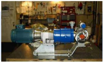
Following our initial success, ROTAN® pumps have been placed in more aggressive service where sulfur is delivered under higher pressures and burned in the production of Mercaptan. Mercaptan is used as an odorant within natural gas and used in the production of plastics. In this service, stainless steel materials were required along with tungsten carbide bearings and thrust washers. Following success here, the same ROTAN® model was chosen within a sister plant operation.
