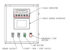
In addition to the Color Touch Screen Operator Interface, mechanical switches for frequently used functions are also provided:
