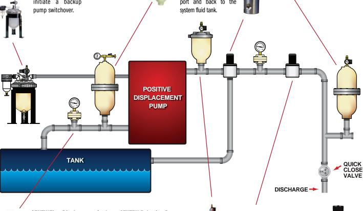
SENTINEL Diaphragm Seals employ a chemically resistant diaphragm to effectively isolate process fluids from gauges and
