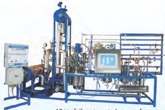
10 Ltr. fully automated ex-proof alkoxylation pilot plant
