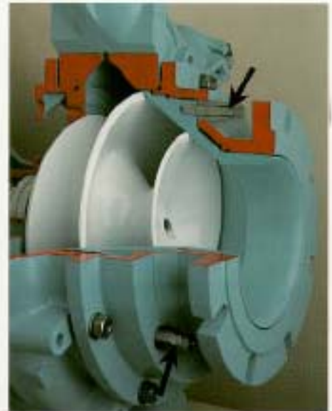
Optional liner easily adjusts for wear with external regulator screws.
